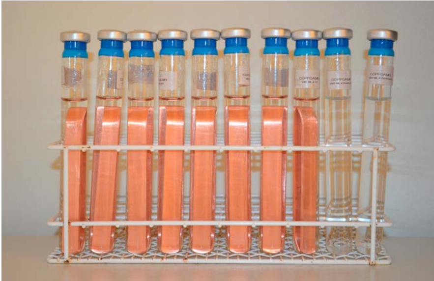
Figure 4-2. Pairs of copper pieces immersed in pure water; contained in butyl rubber sealed borosilicate glass tubes. The 6 cm 3 gas phase at the top is sampled and analysed at regular intervals. Two tubes contain only water and gas. The image was taken after 27 months of exposure to pure, oxygen free water at 70 °C. (Johansson et al. 2015)
