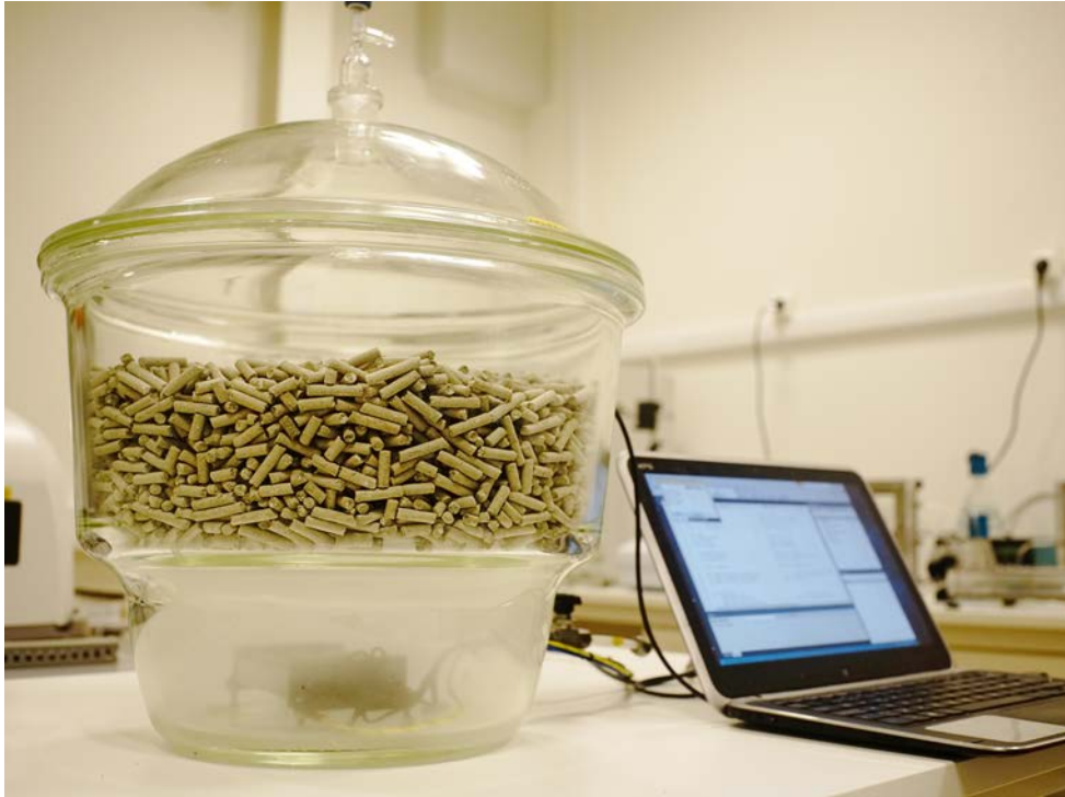
Figure 2-10. Test containing bentonite pellets in a desiccator, heated from below, regulated with a temperature probe in the pellets, and also containing a flask with a solution of divalent copper ions to capture any hydrogen sulphide formed.
