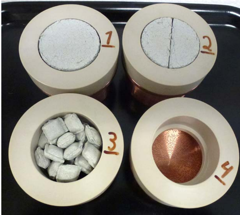
Figure 3-7. Photo showing the four different test types included in all test series: 1. Block, 2. Fractured Block, 3. Pellets and 4. Reference. (Åkesson et al. 2019)
